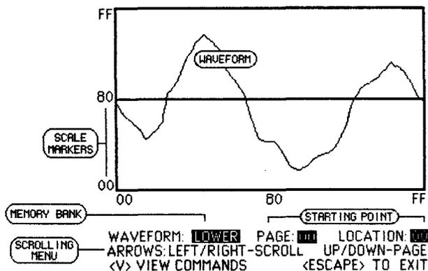
This is the first page of the lower waveform presently in the Mirage. Markers along the vertical and horizontal axes indicate minimum (00), midscale
