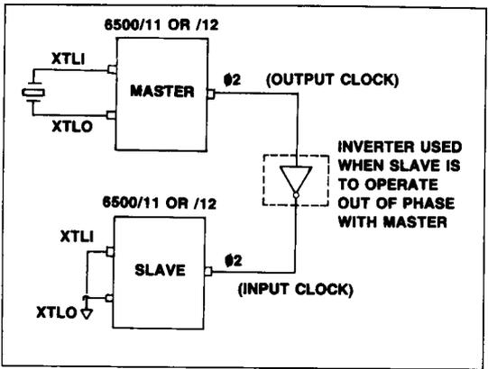
Figure 3-4. Master/Slave Connections
