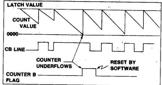
Figure 6-4. Counter B Retriggerable Interval Timer Mode
